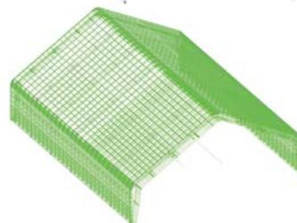
ENVELOPE LOADING D+CL+WIND PARALLEL+IP CONDITION
