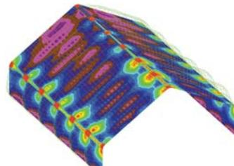
FABRIC STRESSES AND SCALED DISPLACEMENT
